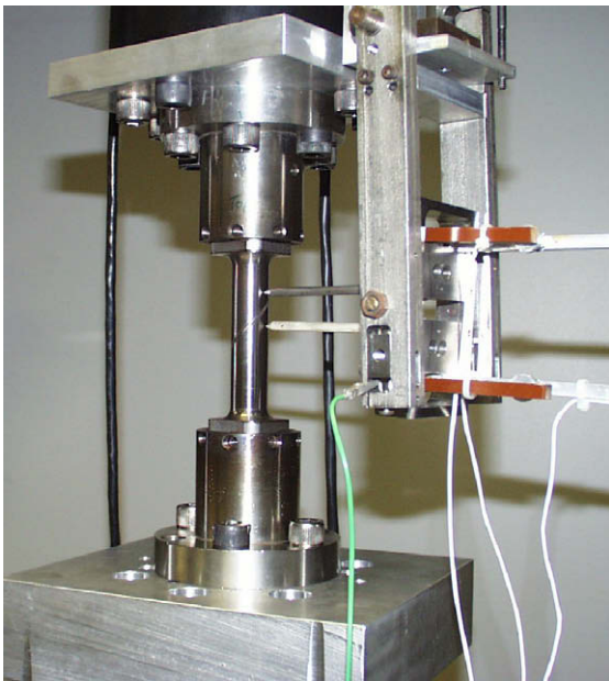
Fig. 1. SNTT test set-up.
