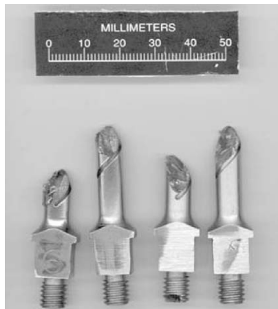
Fig. 15. Fractured MA956 SNTT samples.
